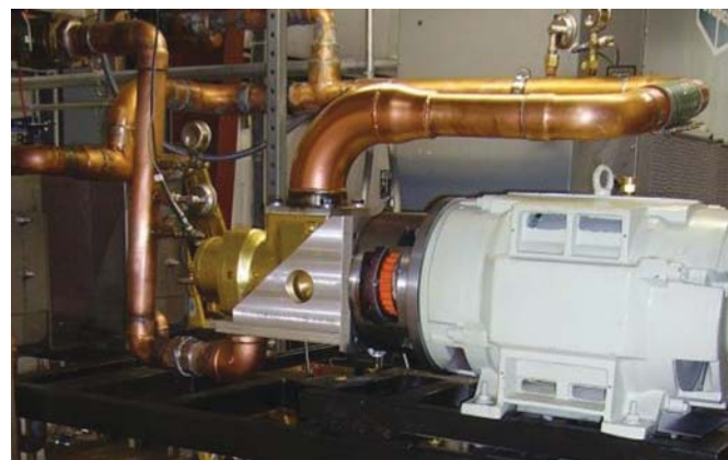
At heart, ElectraTherm's fuel free power systems couples an expander (similar to a turbine) to a generator. Power is fed to an existing grid.
